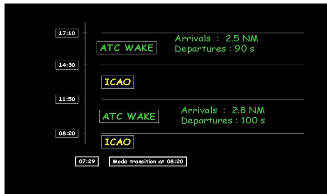
Figure 46 – Supervisor SMP HMI
