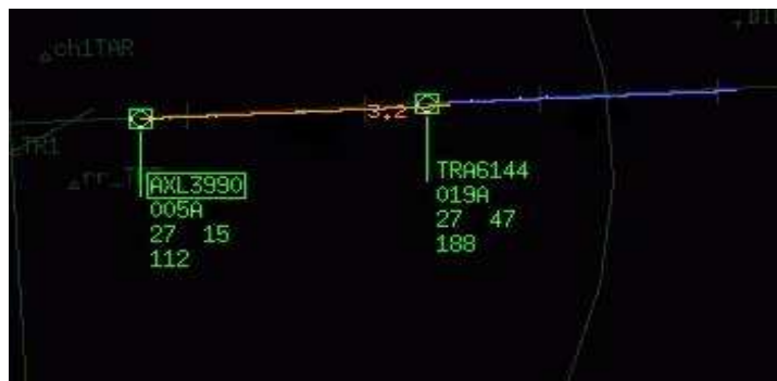
Figure 15 – ATC-Wake alarm for Tower controllers
